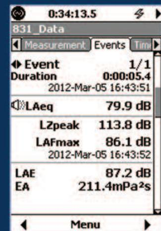
Fig. 22 Event Detection Display on Model 831
